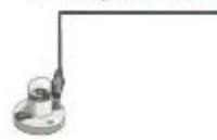
There is a break in the **circuit** that prevents the **electricity** from flowing. The components will not work.
